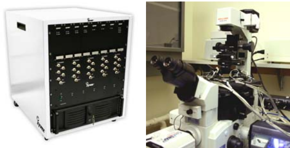
Figure 2 Compact L200 control cabinet, 27" H x 21" W x 26" D (left). L200 installed on a Nikon TE2000 inverted confocal microscope (right).
