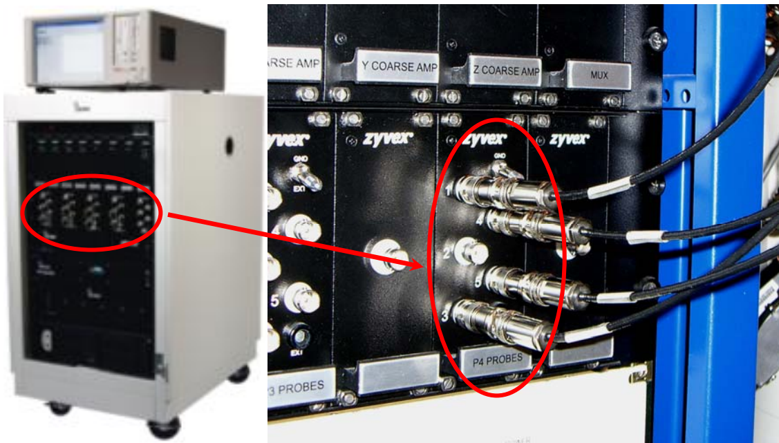
Figure 5. Electrical connections on the front panel for FCP measurements.
