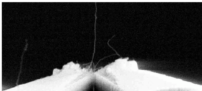
NanoEffector Microgrippers grasping a carbon nanotube bundle.
