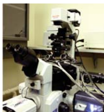
Figure 1a (left) L200 installed on a Nikon Model TE2000 inverted microscope.
