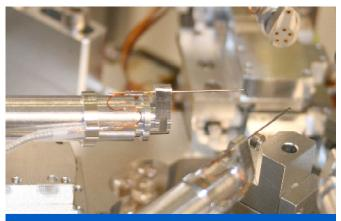
The low noise traixal cable attaches directly to the probe and provides superior electrical performance.
