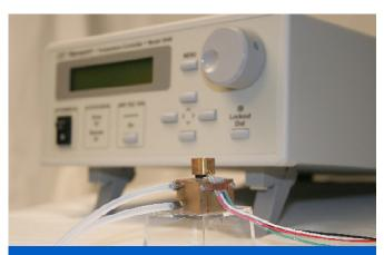
Zyvex Temperature Characterization package includes a high accuracy controllers and a removable thermal sample stage.
