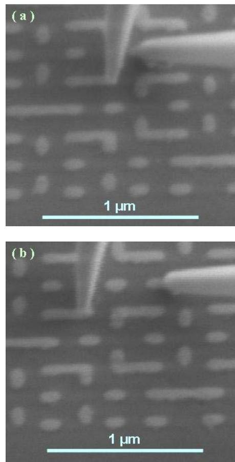
FIGURE 2. Probes touching down on the contacts for C-V measurement, (a) PMOS and (b) NMOS of Intel<sup>TM</sup> 45nm SRAM at metal-0
