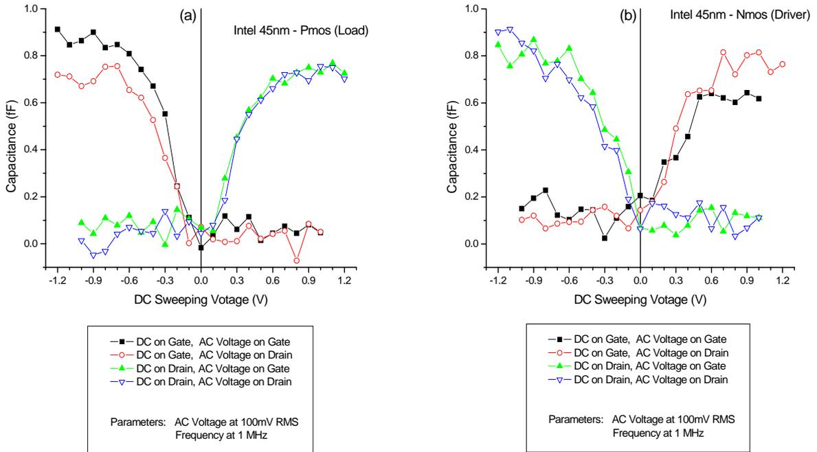
**FIGURE 3.** Capacitance response of the gate of a) PMOS and b) NMOS while applying DC and AC voltages to gate and drain in the following configuration order: gate only, gate and drain, drain and gate, and drain only.
